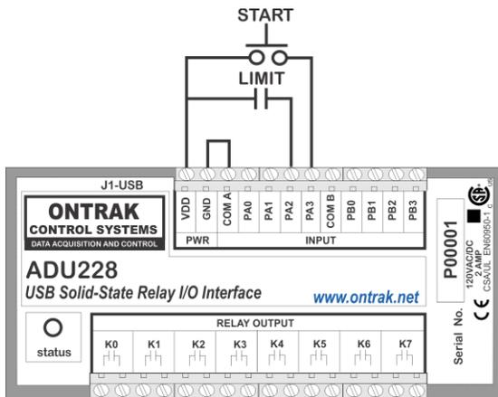
Figure 6A: Dry Contact Connections Using Internal VDD Supply.
