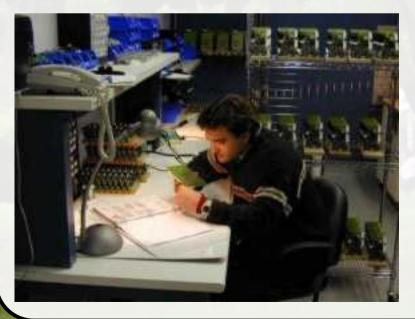
Ontrak's manufacturing facility is well equipped with two through-hole solder lines and one SMT line. Nine CNC mills for enclosure manufacture facilitate complete product development. An in-house CE certification lab ensures a rapid product certification process.
